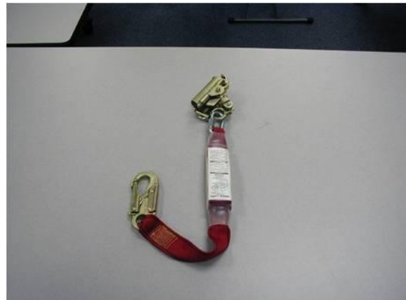
Rope grab – with shock absorber
