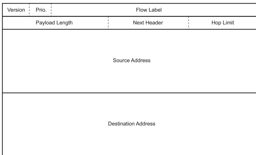
Figure 3 IPv6 Header Format
