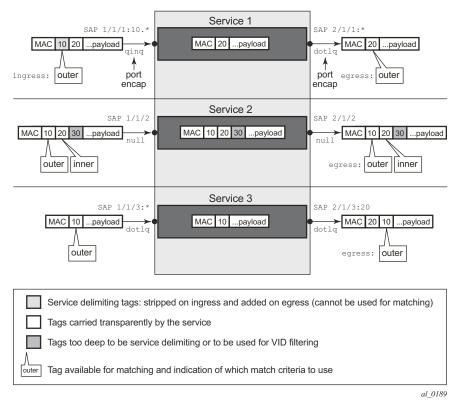
Figure 16: VID Filtering Examples
