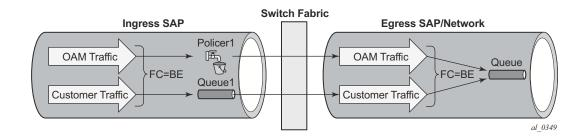
Figure 15: Ingress Criteria Classification Directly to Policer
