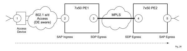
Figure 13: DEI Processing Ingress into the PE1 SAP
