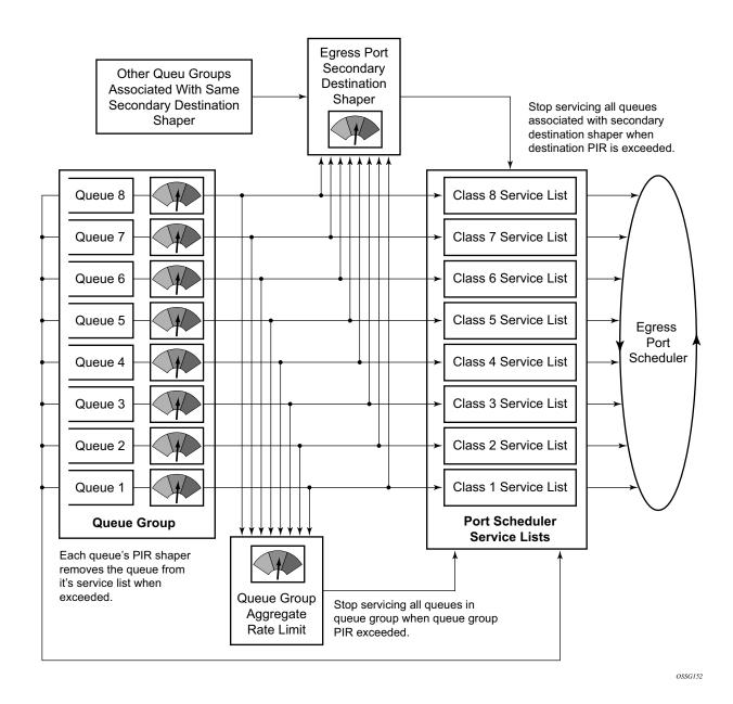
Figure 43: HSMDA Egress Queue Group and Secondary Destination Shaper Behavior
